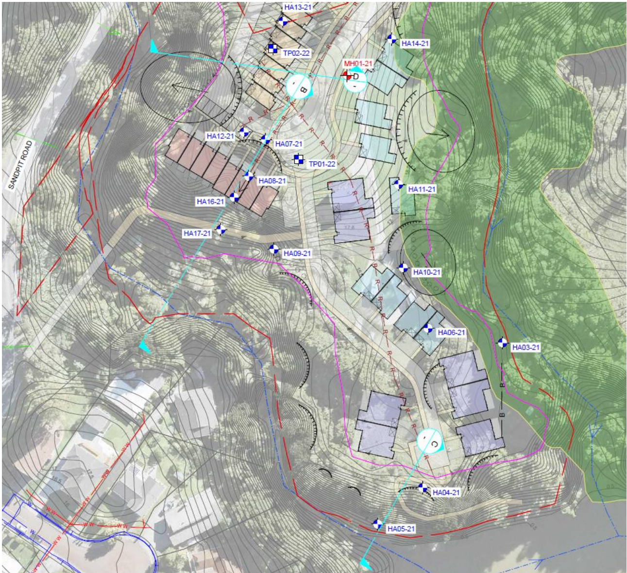
Figure 41. Geotechnical investigations 'as completed' with scheme plan overlaid (detail from CMW Geosciences Ltd March 2022)
